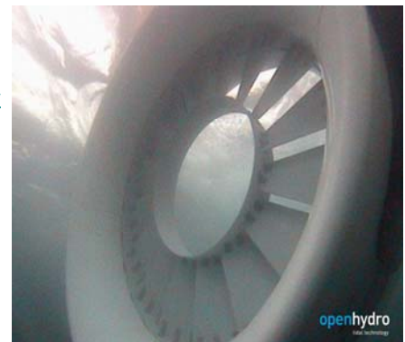
OpenHydro's turbine installed at EMEC.
