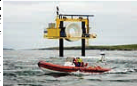
The OpenHydro turbine raised out of the water at the EMEC tidal testing site.
