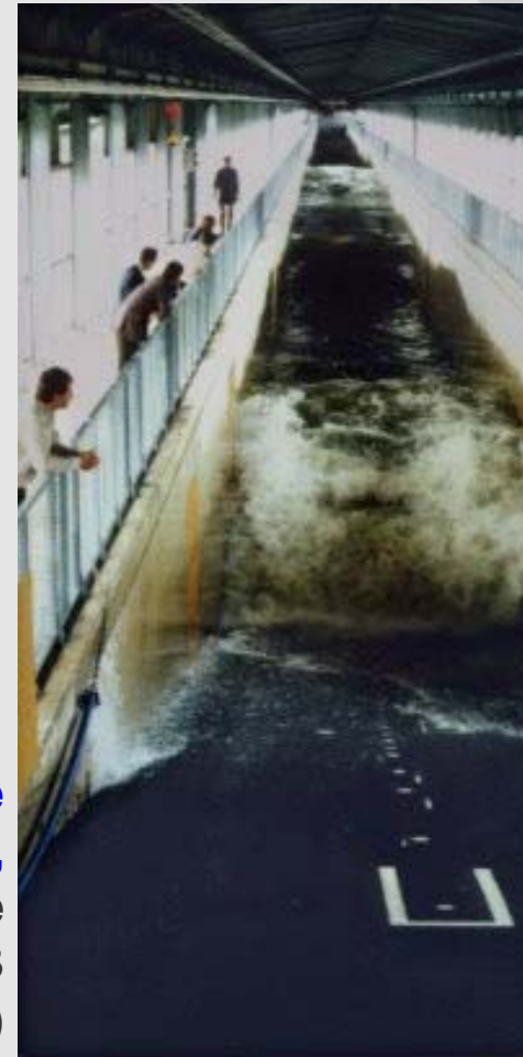
Coastal Research Centre (FZK), Hannover, experimental work in the large wave tank (HYDRALAB I, II, ...)
