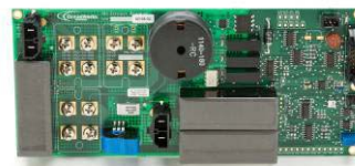
Power Distribution and Breakers
